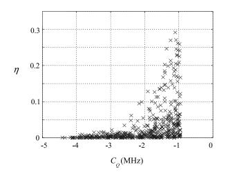
Figure 2: NMR parameters for dataset; structures with larger magnitude  $C_Q$  and smaller  $\eta$  are similar to anatase, while structures with smaller magnitude  $C_Q$  and larger  $\eta$  are similar to rutile.
