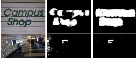
Figure 4. Comparison of the multi-scale, shared-net FCN with a single branched FCN. Left: input image. Middle: single branched FCN. right: shared-net, multi-scale FCN.
