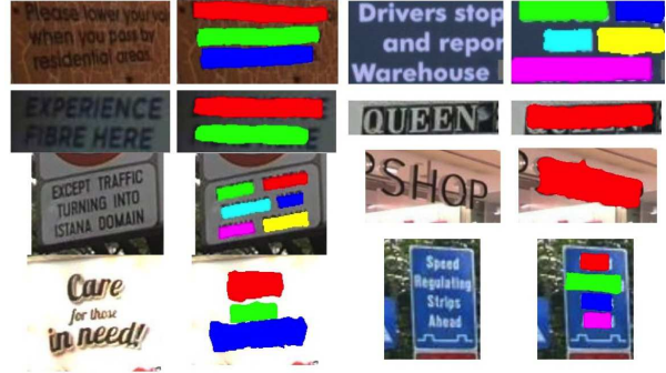
Figure 5. Results of our instance segmentation model. It can capture word or text line instances in a wide variety of circumstances with arbitrary orientations. The segmented results could be directly thresholded to get the final bounding boxes.
