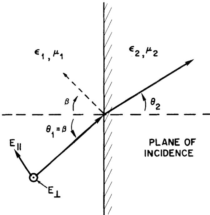
Fig. 1. Incident polarizations, media permittivities and permeabilities, angles of incidence and refraction, and Brewster angle are defined.
